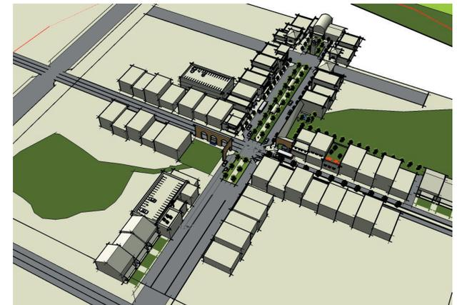
Note the bus right-of-way, a tree-lined boulevard, natural areas connected through the urban area, and large pedestrian sidewalks.
