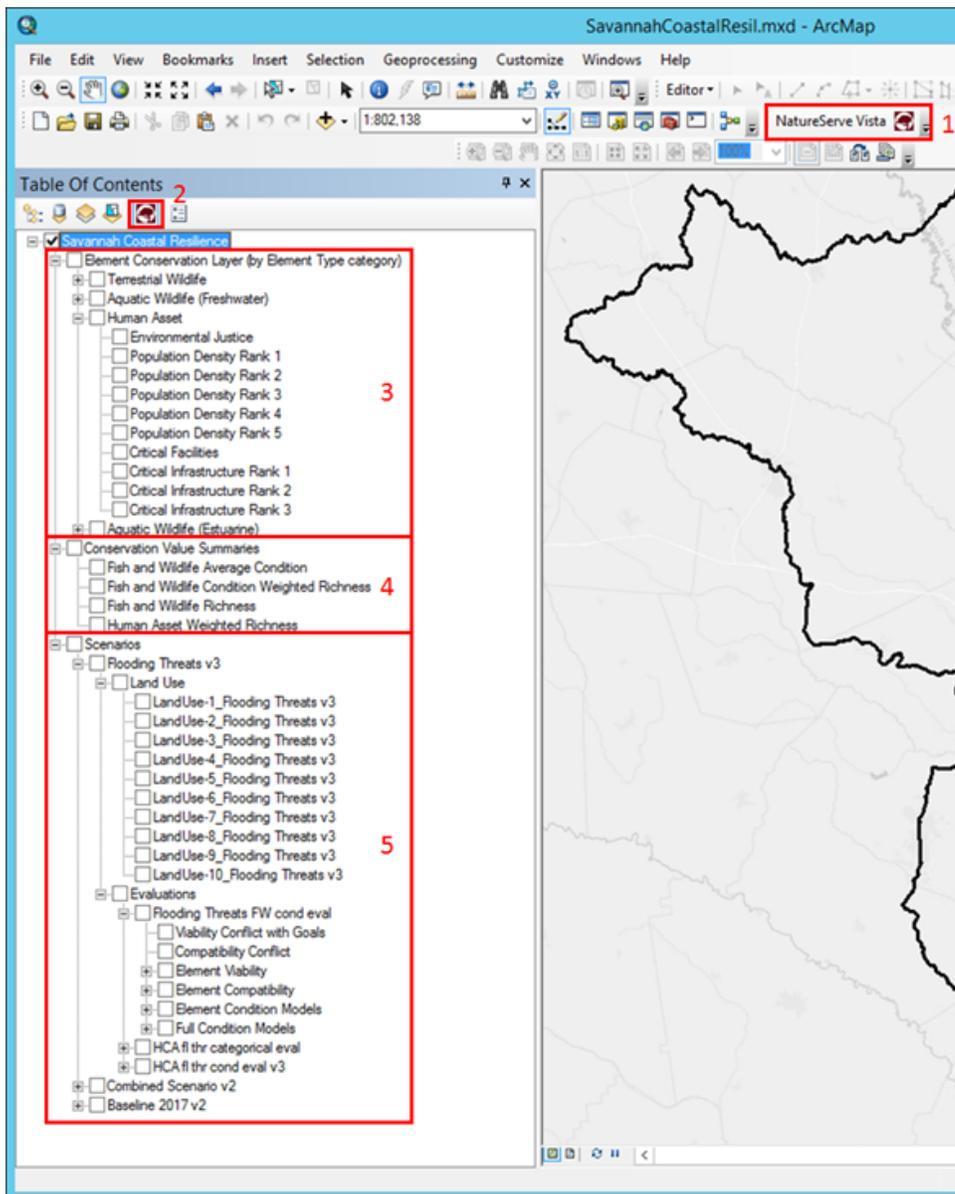
1. The NatureServe Vista toolbar contains the menus accessing all the tool's functionality (it should load automatically when you install Vista but if not, make sure the Vista extension is selected).
